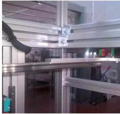
Linear guidance system with ball bearings for centesimal precision
