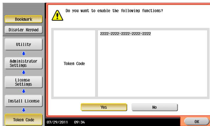
This machine establishes communication with the License Management Server, and enables the advanced function managed by the token number. When the license registration and advanced function enabling steps are ended normally, this machine restarts automatically.
