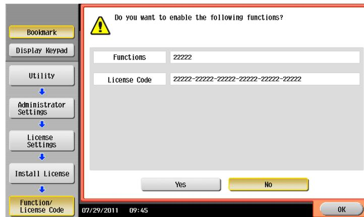
The target advanced function is enabled on this machine. Then, this machine restarts automatically.
