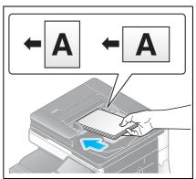
3 Slide the Lateral Guide to fit the loaded original.
