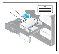
3 Slide the **Lateral Guide** to fit the size of the loaded paper.
