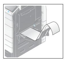
4 Slide the **Lateral Guide** to fit the size of the loaded paper.
